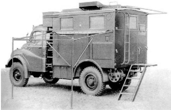
The main penthouse is supported on a folding tubular metal frame that attaches to the vehicle. The frame at the rear of the vehicle is now unfolded beneath this the rear platform and metal ladder have been installed.
