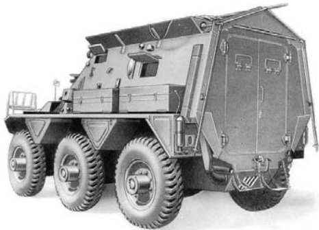
Extendable frame on the much taller Armoured Command Post (FV610).
