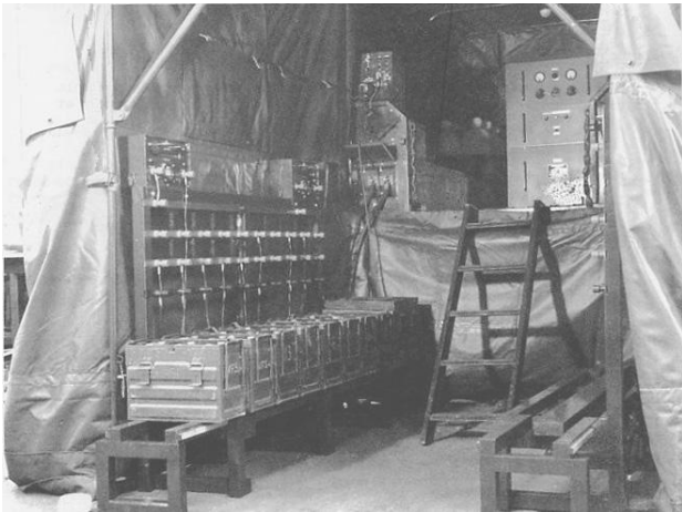
Rear view of the shelter showing batteries on charge.
