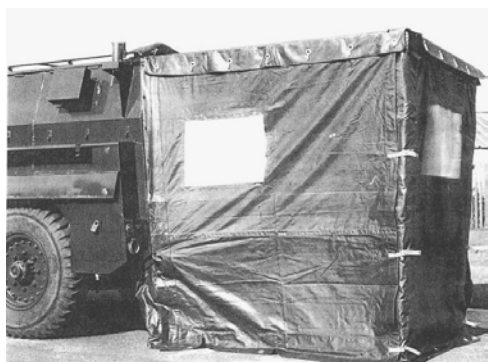
The sidewalls are hooked into eyes on the roof piece.
