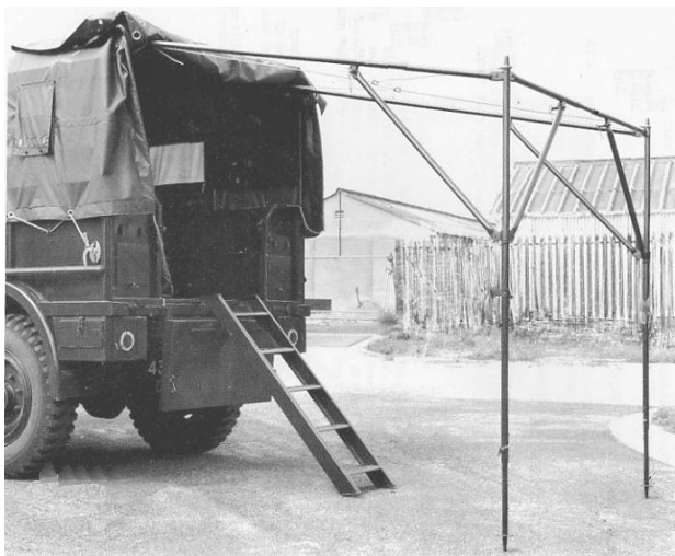
Shelter frame with telescopic legs and folding stays.
