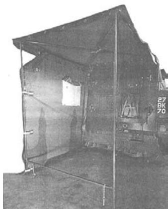
Rear sides attached to poles with straps and buckles.
