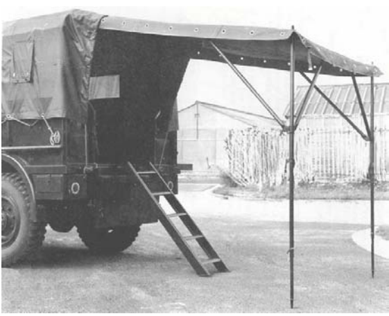
Canopy in position tucked under the vehicle canvas.
