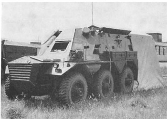
FV610 with penthouse at the rear and at the side of the vehicle. The rear shelter can act as a corridor to interconnect two vehicles.
