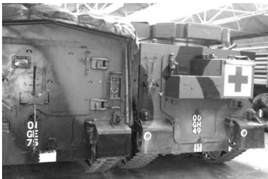
Sultan on the left with shelter and frame. Samaritan on the right, which in the end was not equipped with a shelter.
