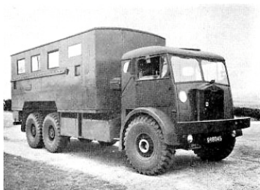
Truck, 10-Ton, 6x4, GS, (Albion) Machinery RE (FV11102)
